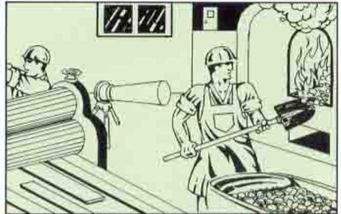
高溫工作環境抽風 VENTILATION FOR WORK FIELDS IN HIGH TEMPERATURES
