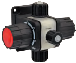
MF MULTIFUNCTION VALVE Multifunction valve (pressure, safety, antisiphon and bleed) 1/2" connections for different hoses diameters. FKM B or EPDM o-ring. PVDF body.
