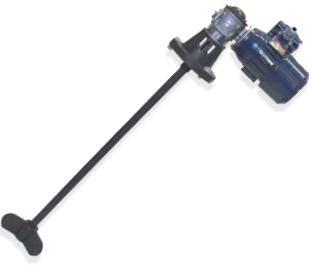
MIXN/8 Slow speed mixer 70/200 RPM. AISI shaft-PVC coated, different lengths available (630-730-830-930 mm). 3-blade impeller, diameter 150mm.
